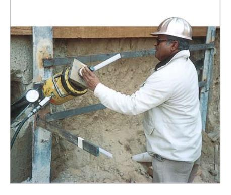
• Immediate pull testing of helical tieback anchors after installation serves as a check on design procedures and eliminates deflection at working loads.
